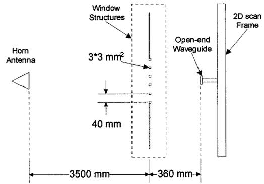
Fig. 11. Layout of scale-model test set. Photograph of the 2-D scanning frame is shown in Fig. 12.
