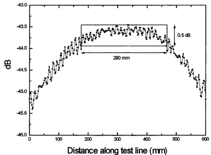
Fig. 14. Calibration test results of horn antenna.
