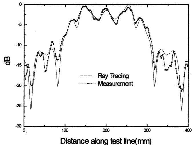
Fig. 15. Comparison of measurement and ray-tracing results.
