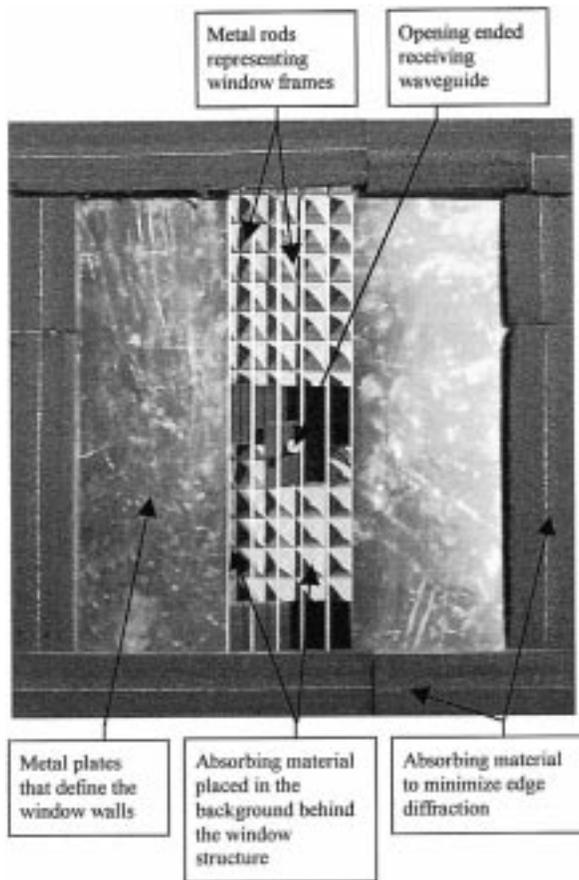
Fig. 13. Photograph of window structure scale model.
