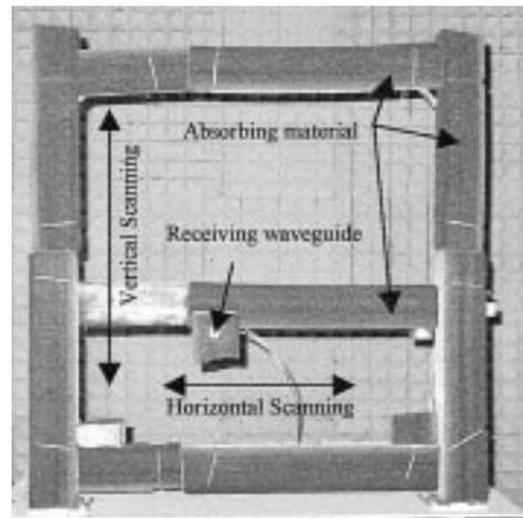
Fig. 12. Photograph of 2-D scanning test frame.
