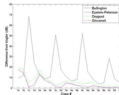
Fig. 1. Difference of diffraction loss models from Vogler.
