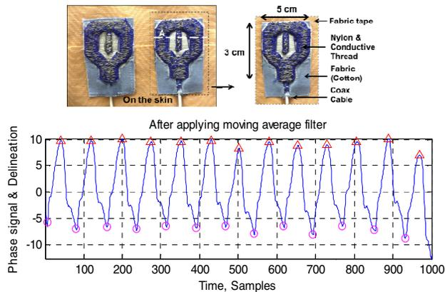
Fig. 1. The fabricated sensors and detection of characteristic points of CPS phase signals corresponding to cardiac activities. Peaks are marked with triangles and valleys are marked with circles.
